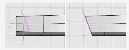
The transom edges do not form a closed boundary. We will add a line to fill the gap for creating the transom surface.
