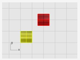
3. On the **Transform** menu, click **Rotate**. *Optional:* Review the Help topic for the Rotate command in Rhino Help. 4. in the Top viewport at the **Center of rotation...** prompt, with the **End** object snap on, click the lower left corner of the half-cylinder as shown in the illustration below.
