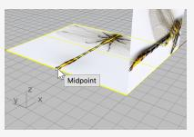
3. Drag the Picture plane, snap to the lower-left corner of the other Picture plane, and release the left mouse button.
