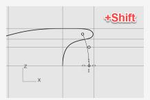
**Note:** Holding down **Shift** enables **Ortho** mode. The second and third points are placed along the y-axis.
