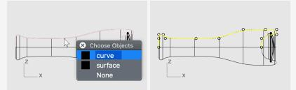
**Note:** When you select a single curve, its control points turn on automatically. The control points turn off when you deselect the curve. If you need control points to stay on when a curve is deselected, select the curve, and press **F10**.
