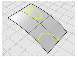
If you have a trimming curve that runs across a surface, the trimming curve itself does not have any real relationship to the control point structure of the surface. You can see this if you select such a trimmed surface and turn its control points on. You will see the control points for the whole underlying surface.
