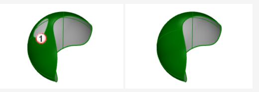
The hole edge is deleted causing the hole to be removed.
