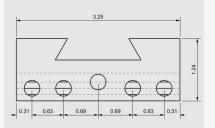
**Note**: If the dimension text and arrows do not fit inside the dimension lines, you can fix this later in the dimension Properties. Dimension properties let you specify the location of the text and arrows.
