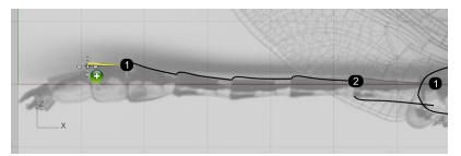
8. Click at the end of the last body segment, and press the **ESC** key to end the command.
