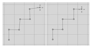
Ortho off (left), Ortho on (right)
