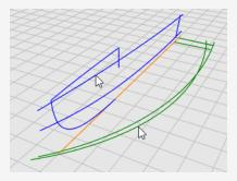
On the Curve menu, click Curve from 2 Views to start the Crv2View command. A 3-D curve is created. It is the intersection of the two surfaces extruded from the two input curves.
