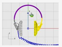
4. At the **End of mirror plane** prompt, turn on **Ortho**, and drag the mirror line straight up and pick.
