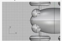
3. Move the cursor to the **Front** viewport, drag the cursor upwards near the end of the ellipsoid, and click.
