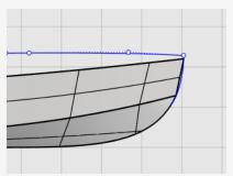
2. Drag the first control point, using the **End** object snap to move the point to the corner of the hull, and click.
