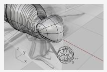
3. Tune on **Gumball** and drag the **Z scale handle** (the small blue rectangle) up to squeeze the sphere into an ellipsoid.
