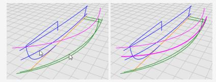
5. When you are satisfied that the proper curves were created, delete or hide the four input curves of the **Crv2View** command.
