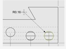
4. Double-click the radial dimension text, and in the text edit box, add the text: **Typ. 5 Places.**
