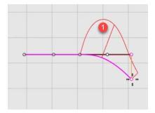
• Conversely, when the curve is bending upward, the curvature graph will be below the curve. (2)
