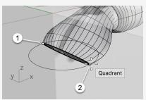
4. In the command options, select **None** for **Direction Constraint** and check **Both Sides**.
