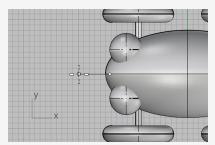
Planar mode keeps successive points at the same construction plane elevation. Elevator mode and object snaps override Planar mode. Watch the curve in the **Front** and **Right** viewports.
