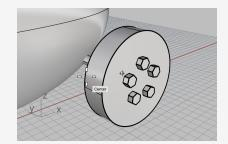
Move the cursor near the other edge until the Cen tooltip appears and click. This places the center of the torus at the middle of the hub "between" the centers of two circles that make up the edges of the wheel hub.
