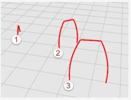
**Tip**: Select the curves by picking near the same end where the numbers are. This avoids twisting the loft surface. In this model, you can use any selection method. The Loft command will sort out the order of the curves. In other more complex cases, picking the curves near the same end may be important, and you may have to make adjustments for the loft to work properly.
