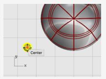
4. At the **Reference point for scaling and rotation** prompt, pick any point to the right or left of the eye ellipsoid.
