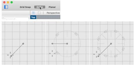
Ortho off (left), Ortho 90° (center), Ortho 45° (right)
