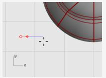
5. At the **End of second axis** prompt, type **1.1**, and press **Enter** to constrain the distance.
