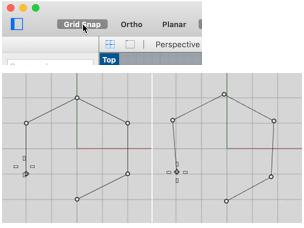
Grid snap on (left), Grid snap off (right)
