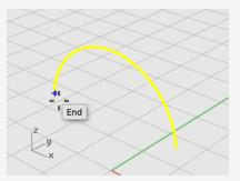
5. At the **Center of ellipse** prompt, snap to an endpoint of the headband curve and click.
