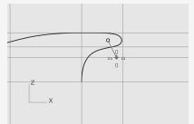
4. For the third point, hold down **Shift**, snap to the lowest guide, click, and press **Enter** to end the curve.
