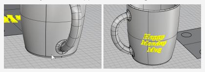
If the base or target surface is not selected at the correct corresponding position, the text objects will be wrapped with a wrong orientation. When it happens, undo the command and try again.
