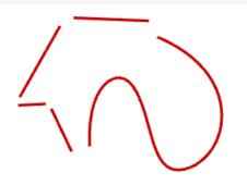
**Note**: For the illustration, the **ScalePositions** command was used to separate the individual curves. The Explode command does not move the curves.
