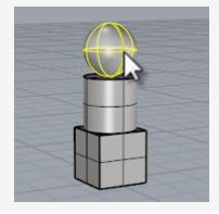
Hold the **Shift** key and select the cylinder. The cylinder is added to the selection.
