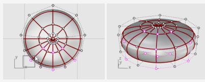
2. Start the **Scale2D** command, and in the **Top** viewport, pick the center point with the **Point** object snap as the **Base point**.
