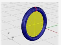
This fills the area at the base of the padding with a planar surface created from the edge of the sweep.
