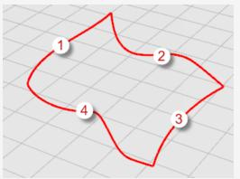
To select the curves, you can click each individual curve using the **Shift** key, or you can use a window or crossing selection to select all of the curves at once. To review selecting objects, see *Chapter 3, Selecting Objects*. A surface is created from the curves, which define its edges.
