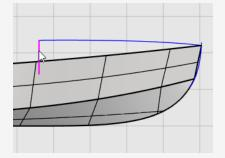
3. At the **Select surfaces...** prompt, select the hull, and press **Enter**. The line is projected onto both sides of the hull.
