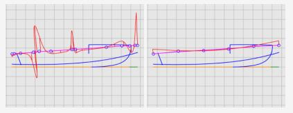
The curvature is improved, but it is not good enough. From the curvature graph, we can tell that the black curve in the right illustration is the real shape of the current sheer curve if we overstate it. It bends three times. We will improve the curve further by editing its control points to make it bend only once.
