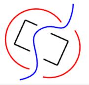
The red circle and the black rectangle are split by the blue curve. **Note**: For the illustration, the individual curves were moved. The Split command does not move the split objects.
