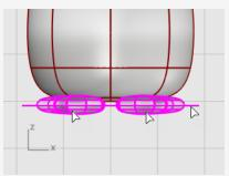
4. While the remaining surfaces are still selected, on the **Edit** menu, click **Join**. The surfaces are joined into two closed polysurfaces.
