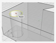
5. At the **Point to copy to...** prompt, snap to the next point that makes the center of the next hole, and click.
