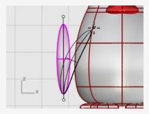
6. If further positioning is required, use **Gumball** to place the wing.
