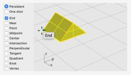
**Note:** In this simple example, you will first show the object's original size by picking two points, a base point and a first reference point. Then you will show the object's new size by picking a second reference point.
