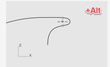
Note: Holding down Alt hides the guides and avoids snapping to the guides.
