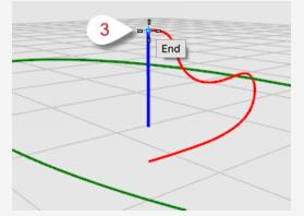
6. At the **End of RailRevolve axis** prompt, snap to the other end of the axis line (4).
