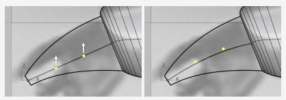
5. In the **Top** viewport, move the two control points in the vertical direction to make an "S" shape.
