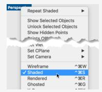
**Note:** The Shaded display mode uses render meshes to display surfaces so you can see the surfaces when they are created.
