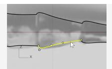
2. Move the control points to make the curve match the image.
