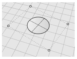
The **Untrim** command removes the trimming curve from the surface to get back to the underlying untrimmed rectangular surface.
