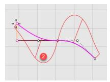
• The point of inflection (where the bending is reversing from one side to the other) is where the curvature graph crosses the curve. (3)
