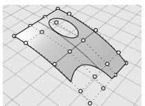
Since it can be important for you to know if a surface is trimmed, the **Properties** command lists the trimmed or untrimmed state of the surface. Some Rhino commands work only with untrimmed surfaces and some software does not import trimmed NURBS surfaces.
