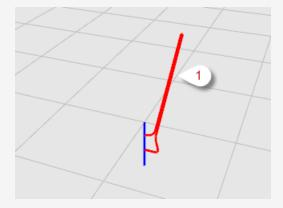
5. At the **Start of revolve axis** prompt, snap to one end of the line (2) that defines the revolve axis.
