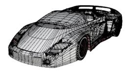
**Note**: There is no easy way to convert a mesh model into a NURBS model. The information that defines the objects is completely different.
