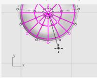
4. Drag the points to make the whole foot about twice the size of the original ellipsoid and click.
