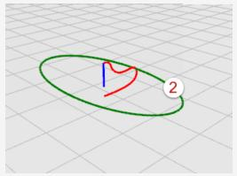
5. At the **Start of RailRevolve axis** prompt, snap to an endpoint of the axis line (3).
