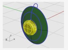
Surfaces that share an edge can be joined into a polysurface. In the next step, you will join all the surfaces.
