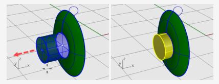
**Note**: The cylinder you just created is an extrusion object (solid). The housing cylinder needs to be open on the bottom.
