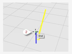
6. At the **End of revolve axis** prompt, snap to the other end of the line (3) that defines the revolve axis.
