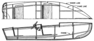
The designer's curves are illustrated. The sheer and chine are extended at the forward and aft ends to accommodate the lofting process.
