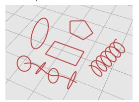
Curves in Rhino include lines, arcs, circles, free-form curves, and combinations of these. Curves can be open or closed, planar, or non-planar.
