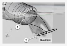
4. In the **Front** viewport, select the curve, and move the two control points up a small distance.
