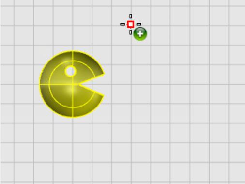
6. At the **End of mirror plane...** prompt, drag the cursor toward the bottom of the screen, and click to end the mirror line.
