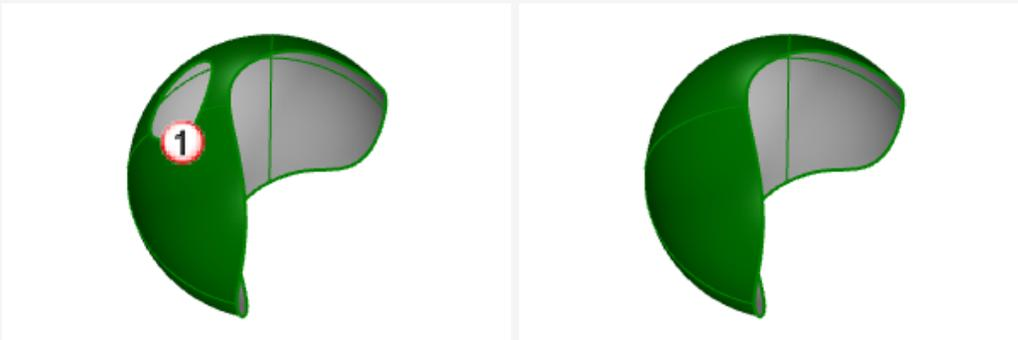
The hole edge is deleted causing the hole to be removed.
