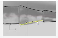
2. Move the control points to make the curve match the image.
