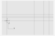
Note: When guides display, Intersect and Near object snaps are always turned on.
