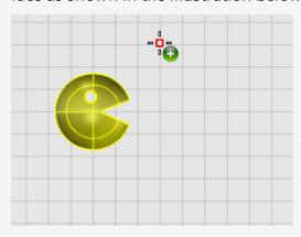
6. At the **End of mirror plane...** prompt, drag the cursor toward the bottom of the screen, and click to end the mirror line.
